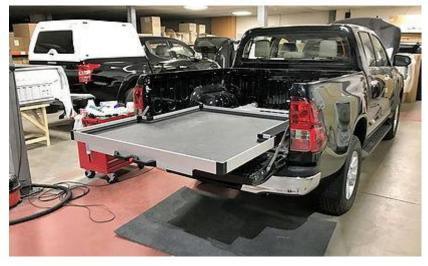
The sliding drawer is particularly useful in the custom version for pickups, providing a massive help in the loading and unloading of the goods, thanks to the extendable corrosion resistant and heavy-duty support. Our product has been tested to support 500 kg load when closed and 250 kg load when extended (up to 70% of its length)
